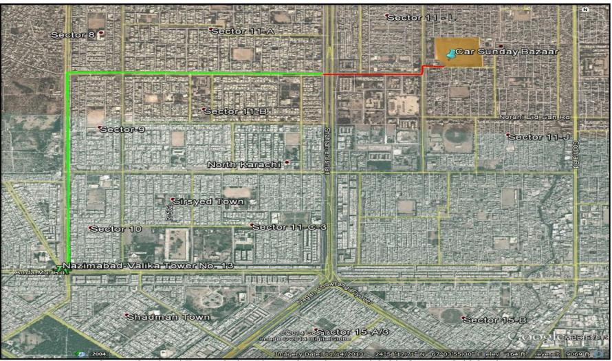
Green: Overhead Transmission Line Red: Underground Cable Orange: Grid Station
